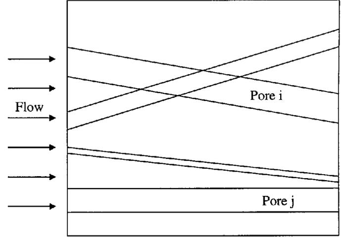
Figure 1: Straight capillary morphology model
