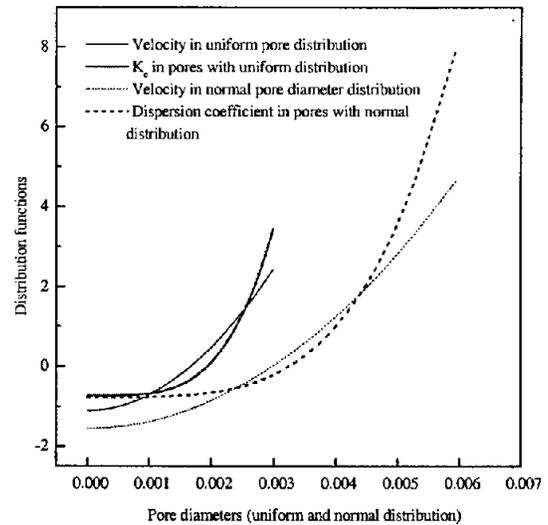
Figure 5: Comparison of laminar regime velocity and dispersion coefficient for straight capillary with normal and uniform pore diameter distribution
