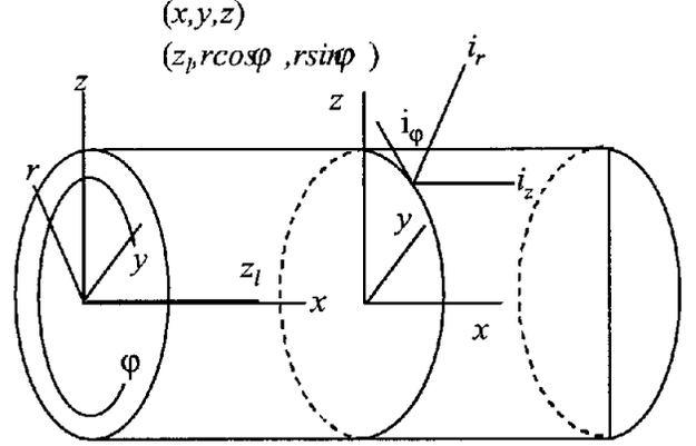
Figure 2: Transformation between upper scale Cartesian coordinate system and pore local cylindrical system.
