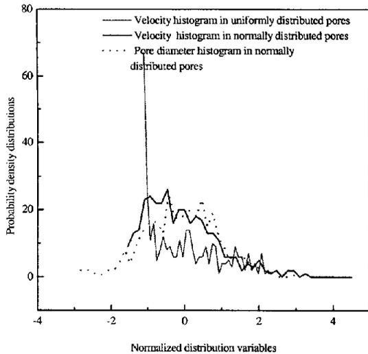
Figure 6: Laminar regime velocity histogram for straight capillary with uniformly and normally distributed pore diameter
