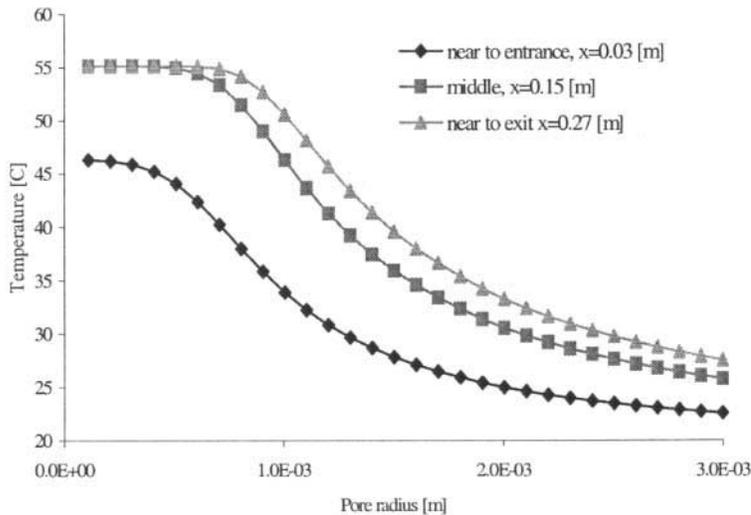
Figure 7: Pore average temperature for different radius pore at different position
